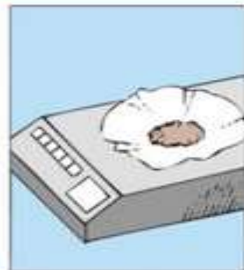
(e) Repeated drying and weighing until a constant mass of precipitate is obtained
